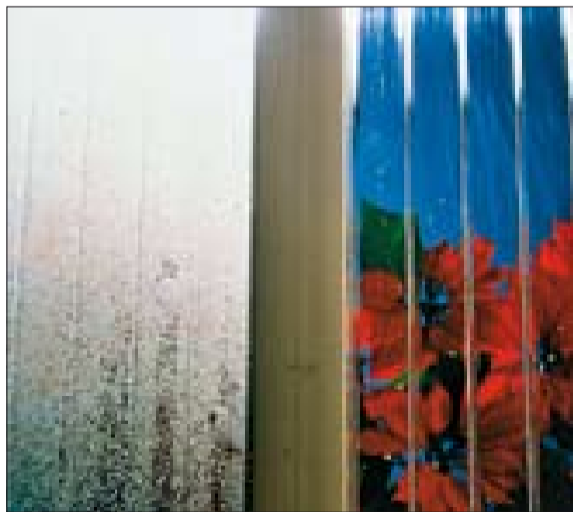
Right: The NO DROP coating applied on both sides and inside the cavities of PLEXIGLAS ALLTOP® double-skin sheets causes water drops to form a continuous thin film. The sheets thus retain their high light transmission. Left: Double-skin sheets without NO DROP coating. Condensation obscures the view and blocks out sunlight.
